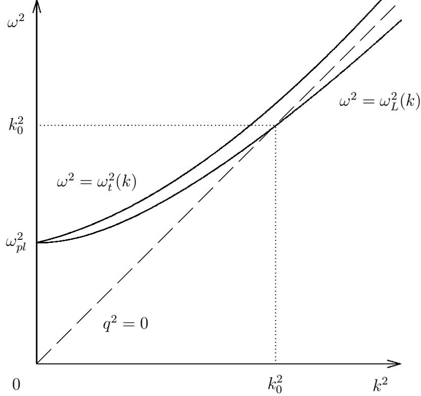
Figure 3: Dispersion curves for transversal plasmon  $\omega^2 = \omega_t^2(k)$  (upper solid line), longitudinal plasmon  $\omega^2 = \omega_L^2(k)$  (lower solid line) and vacuum photon  $q^2 = 0$  (broken line).
